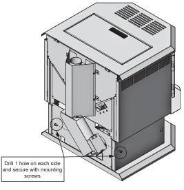
Put a 1/4 inch bead of silicone on the outer edge of the Top Vent Adapter Assembly (C1) exhaust outlet (Figure 5).
