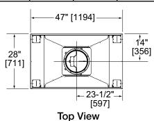
\* Framing must be filled in to top of front standoff after unit is installed.
