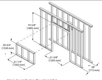
\* Frame down to fireplace after unit is installed. \*\* If the inside of the framed cavity is to be finished, the framing dimensions must include the finished surface. If drywall is to be attached to the rear wall, the depth must be measured from the drywall surface. Add 9-1/4 inches to framing depth for an elbow vented off the rear of the appliance.
