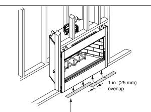
Protective metal strips are placed 2 in. (51 mm) under the front of the fireplace and must extend beyond the front and sides of fireplace opening by 2 in. (51 mm).
