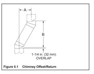
**Example:** Your "A" dimension from Figure 5.3 is 14 1/2 in. (368 mm). Using Table 5.2 the dimension closest to, but not less than 14 1/2 in. (368 mm) is 15 3/4 in. (400 mm) using a 30° offset/return. It is then determined from the table that you would need 36 5/8 in. (930 mm) (Dimension "B") between the offset and return. The chimney components that best fit your application are two SL1112s or SL412s.
