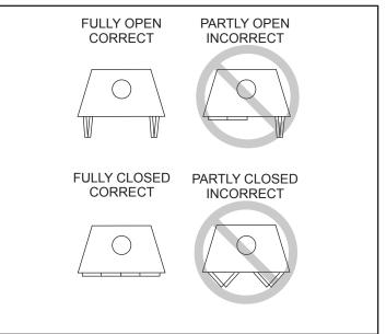
Figure 9.2 Proper Operating Positions of Bi-fold Doors
