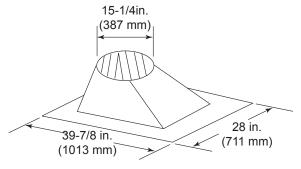
**RF571 Roof Flashing**
