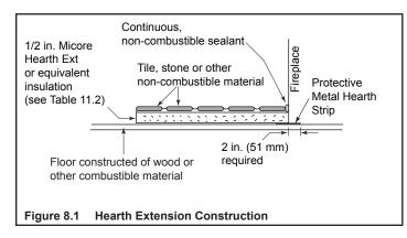
The hearth extension should slope away from the front of the fireplace and chase at 1/8 in. to 1/4 in. per foot. Spark strips must be used on top of any combustible hearth materials used for moisture management.
