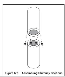
**Note:** Inner flue and outer liner sections cannot be disassembled once locked together. Plan ahead to ensure the proper installation height is achieved with the selected chimney components.
