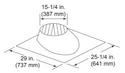
**RF570 Roof Flashing**
