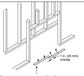
Protective metal strips are placed 2 in. (51 mm) under the front of the fireplace and must extend beyond the front and sides of fireplace opening by 2 in. (51 mm).
