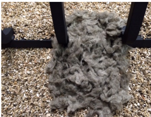
Figure 8c- Carry over tube covered by rock wool
