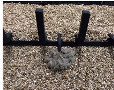
Figure 5b- Packing rock wool around the carry over tube
