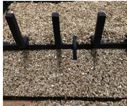
Figure 5b- Packing rock wool around the carry over tube
