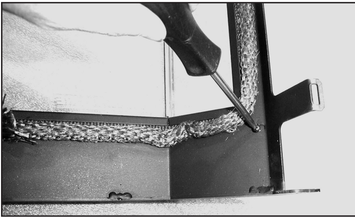
Figure 8.7 - Uninstall the existing crown by removing the four screws on the back side of the door. Retain the screws.
