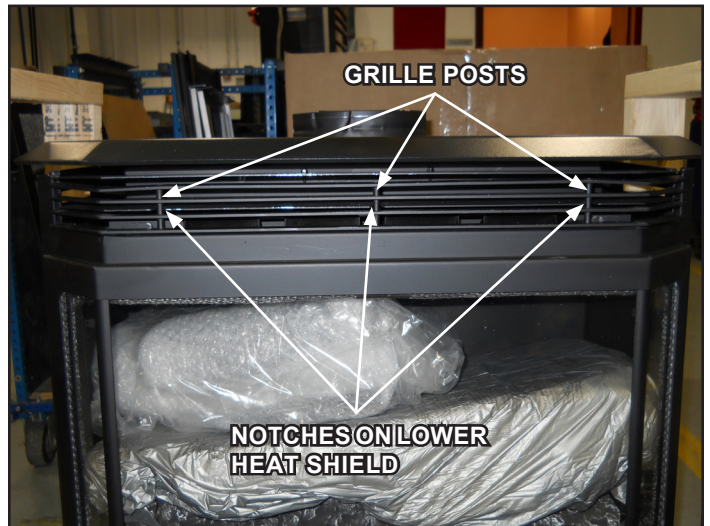
Figure 8.4 - When reassembling the door, be sure to line up the lower shield in the middle grille, line up the grille post with the notches in the lower heat shield. Once shields are lined up (post should be flush with front of shields) push up on the shields using the door and push in to allow the door to rest on the latches. Figure 8.4.
