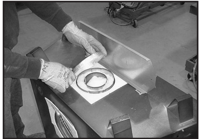
Figure 6.4 Remove the seal cap.
