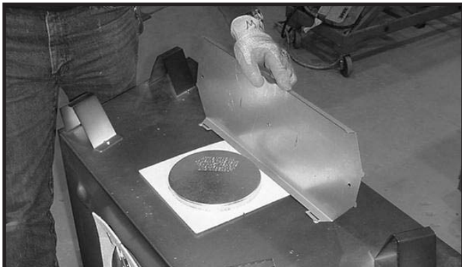
Figure 6.2 Rotate the top heat shield to the vertical position as shown above. The heat shield must remain in the vertical position.
