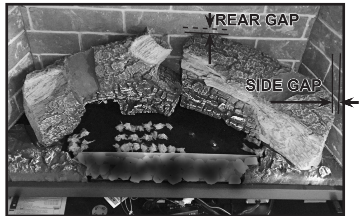
Figure 5. Rear Right Log Installed
