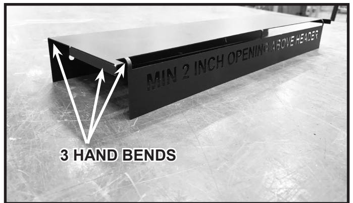
Figure 8.20 All Hand Bends Complete
