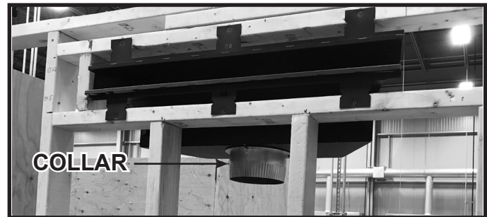
Figure 6.16 Install Collar to Bottom of Plenum
