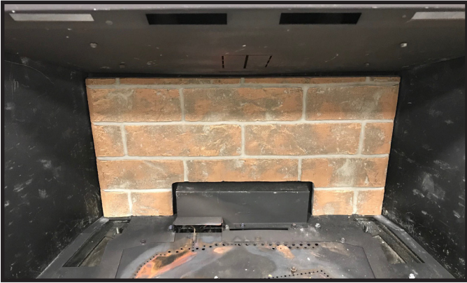
Figure 4 Back Refractory Installed
