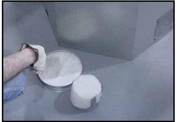
Figure 6.11 Discard the seal cap, remove and discard the insulation basket. Note: Once the seal cap has been removed it CANNOT be reattached.
