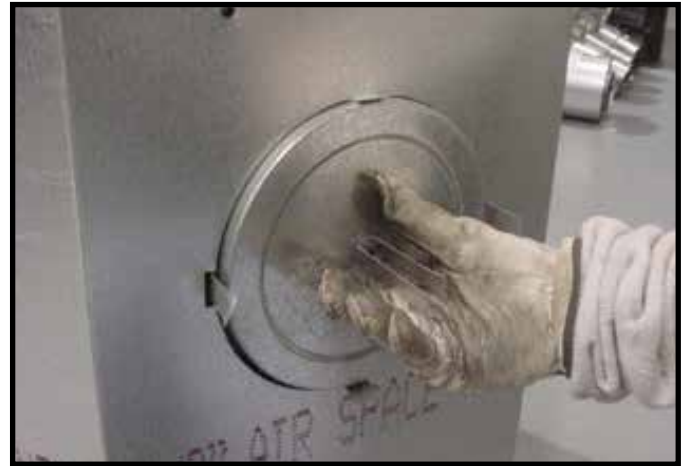
Figure 6.10 Fold the center parts of the retaining band toward the center as shown. Remove the seal cap.
