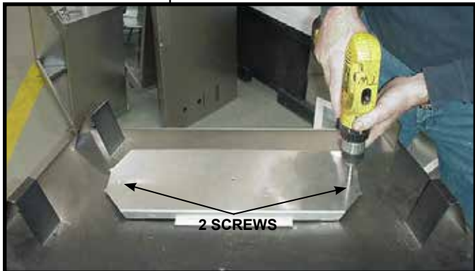
Figure 6.2 Remove the two screws holding the top heat shield in place. For rear vent, see next page.
