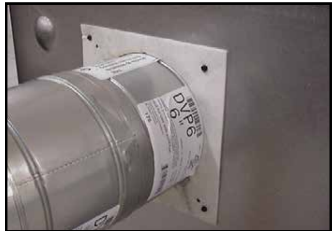
Figure 6.12 Attach the first vent section (it will snap into place). Slide the insulation gasket onto the vent section, up against the appliance and over the tabs. Use four self-tapping screws to secure gasket to outer wrap.
