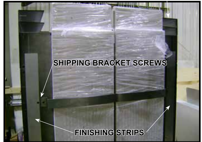
Figure 6.3 Shipping Brackets and Finishing Strip Locations.
