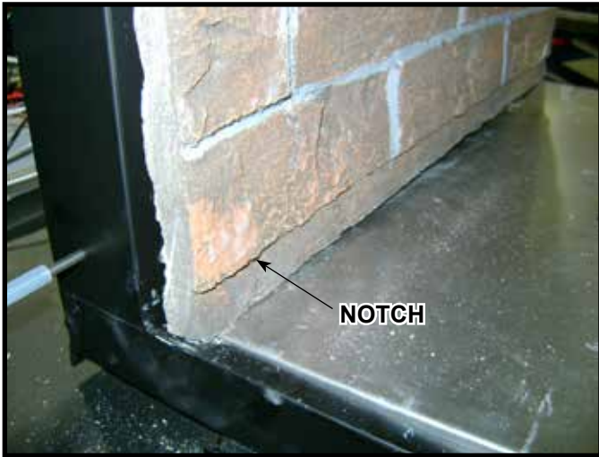
Figure 11.15 Notched End of Side Refractory
