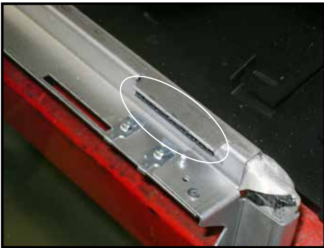
Figure 11.1 Glass Top Tab Detail.
