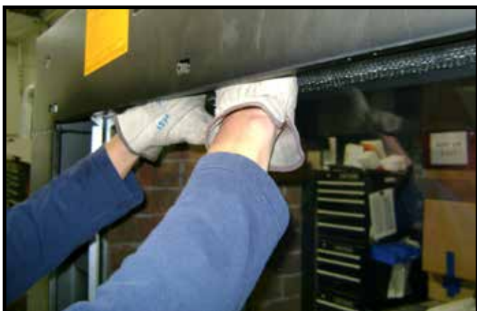
Figure 11.6 Top Glass Latch Access
