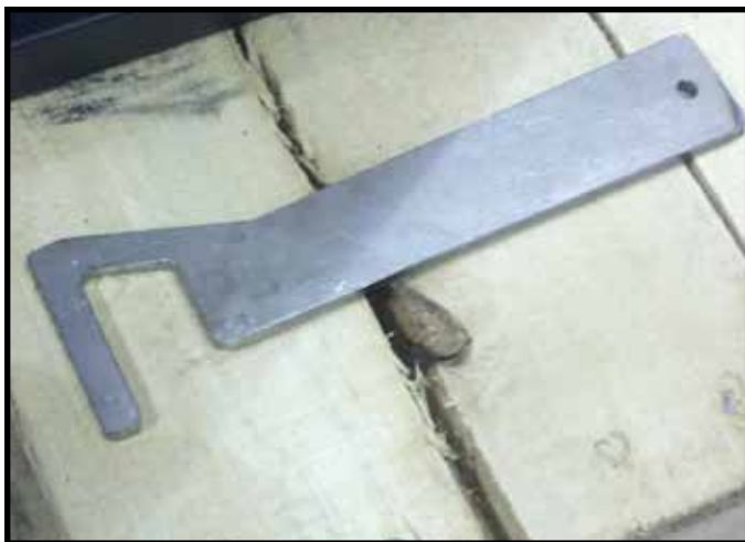
Figure 11.1. Glass Clip Tool
