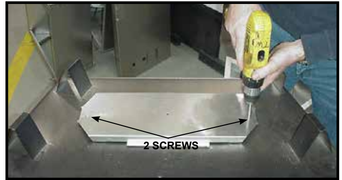
Figure 6.5 For top vent, remove the two screws holding the top heat shield in place. For rear vent, see next page.
