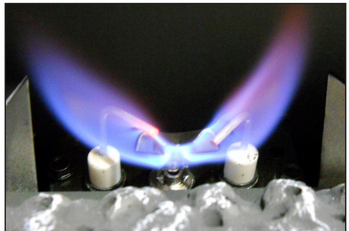
Figure 4.3 IPI Pilot Flame Patterns
