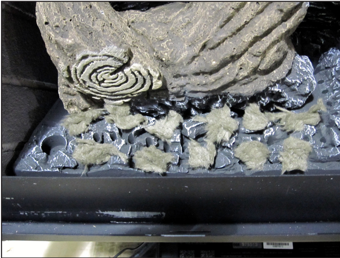
Figure 10.13 - Place Mineral Wool
