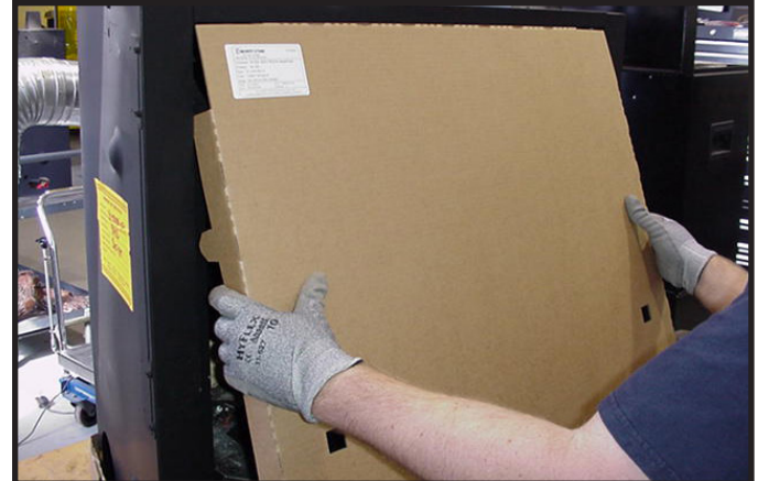
Figure 13.4 Installation of Splatter Guard
