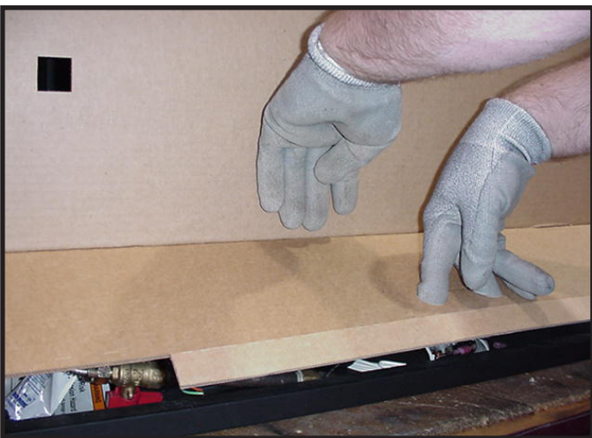
Figure 13.8 Opening Lower Access Panel
