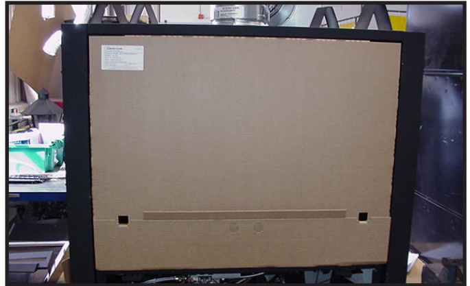
Figure 13.10 Splatter Guard with Lower Access Panel Open
