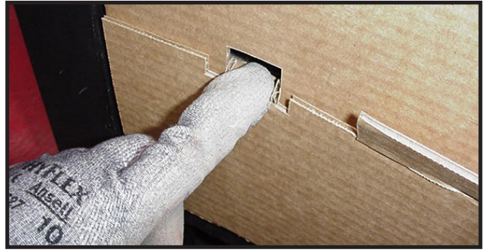
Figure 13.9 Securing Tabs Inside Front of Splatter Guard
